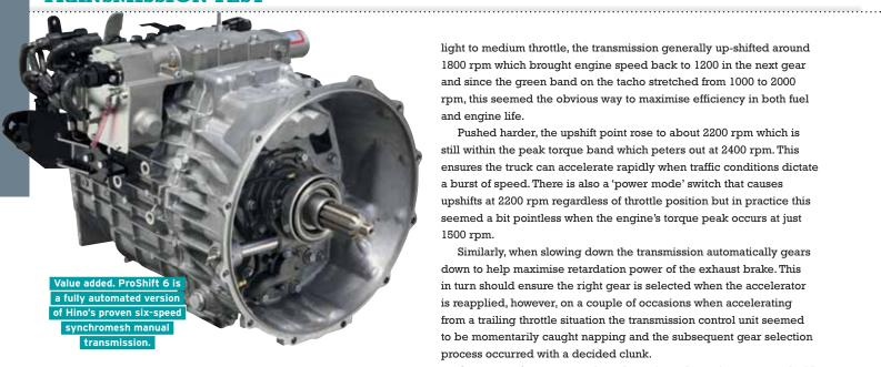
effect of automatic vehicles because a ProShift truck will not move without throttle input from the driver.
