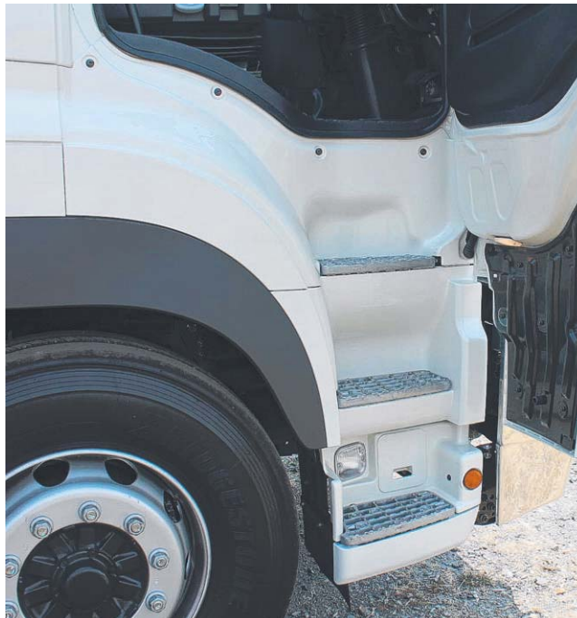
Good-sized steps make accessing the cab relatively easy.
