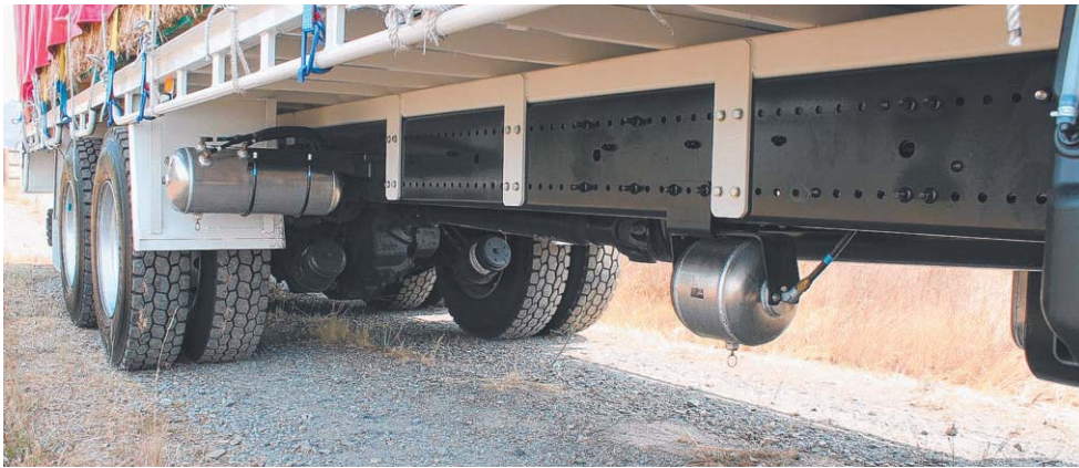
Airbag suspension features on the two drive axles.
