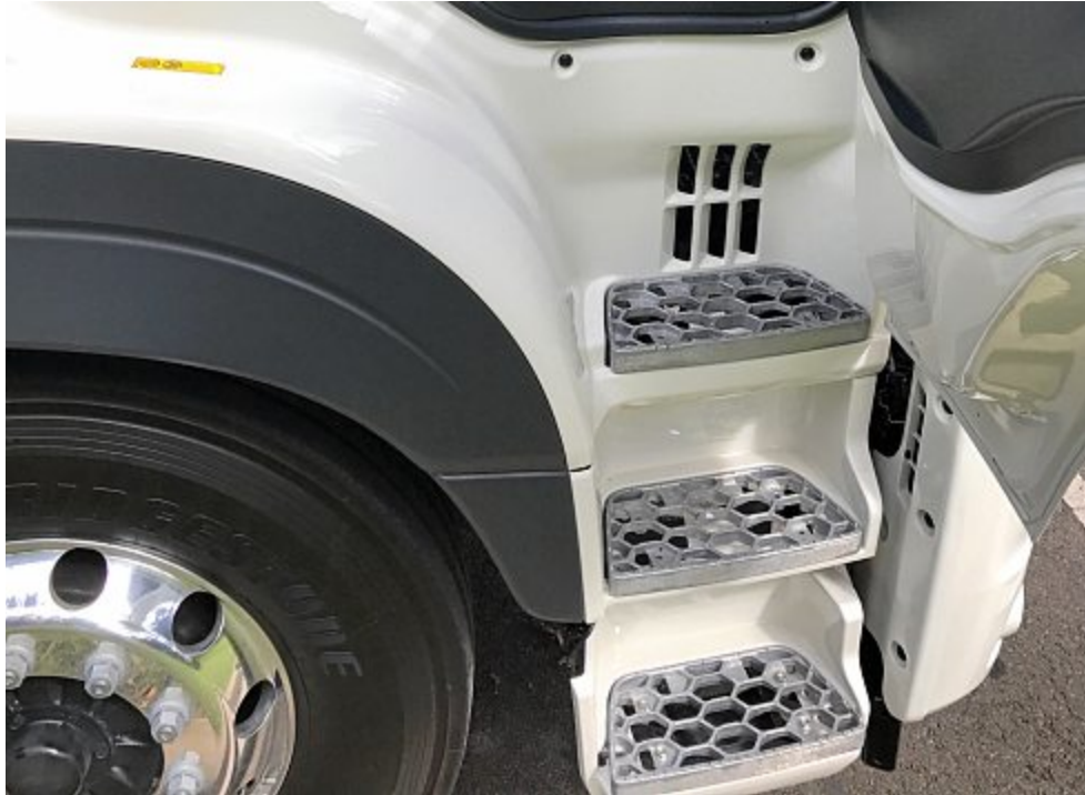
Three steps and swing into the saddle is an easy access for a truck that most likely require a driver multiple exits in a shift.
