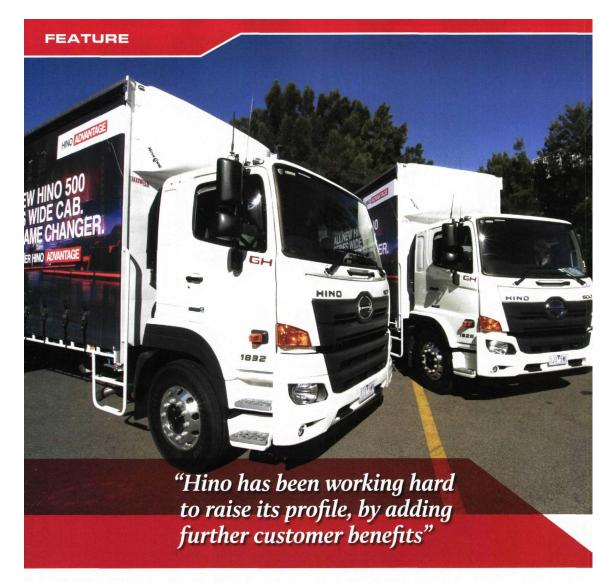
With the 500 Series, Hino is fitting Euro 5 emissions engines using SCR and AdBlue, but without diesel particulate filters that require an occasional engine regeneration.
