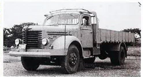
▲ The Hino all-new 1950 TH10 model with a 7 litre engine and 8 tonne carrying capacity.
