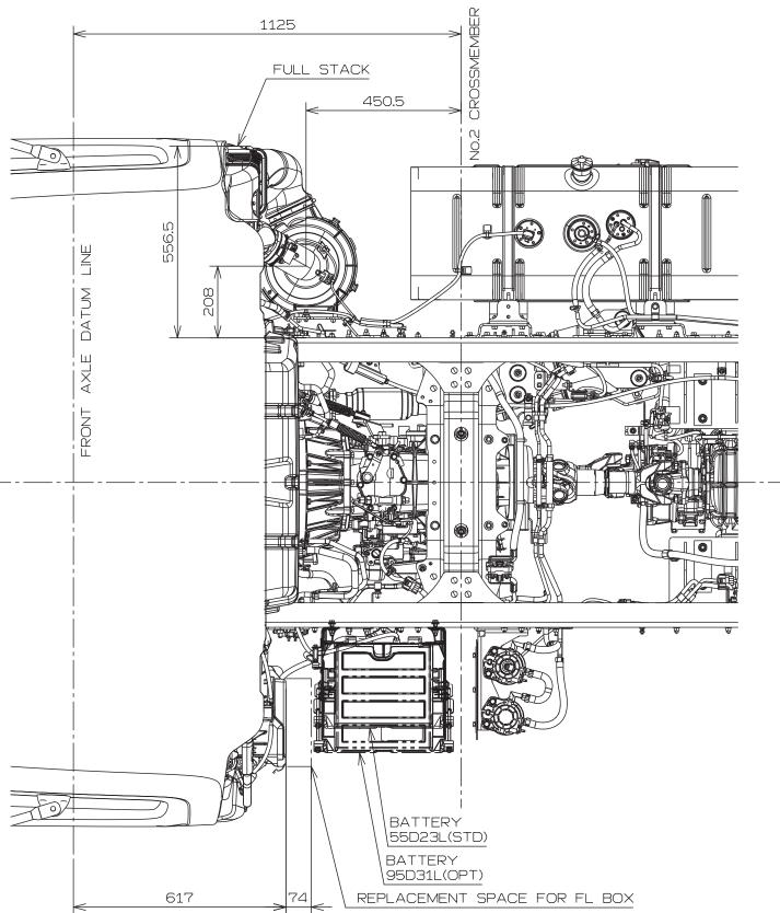
$<sup>\</sup>cancel{k}$  Refer to Chassis with cab drawing for the layout of Fuel tank, Tool box and Spare tire.
